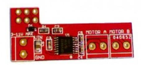
This tiny little board (38 x 16mm) can be added to a Raspberry Pi Zero (or any other Pi for that matter) to provide dual H-Bridge control of 2 DC motors.
