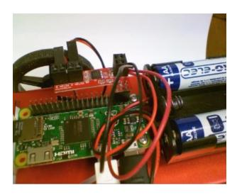
Alternatively, you can mount it by soldering it directly to the bottom of the header, thus leaving the header free to attach other boards as shown below:
