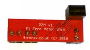
Above shows the PZM with a female header added so it can be plugged onto a "normal" male header as shown below, Note how the PZM sticks out from the Pi, so other boards can still be mounted as usual
